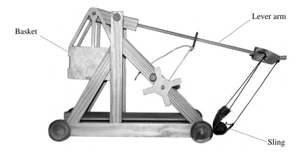
To operate this model, coins are placed in the basket and a small projectile is placed in the sling. When the basket is released, it falls quickly, swinging the lever arm up and shooting the projectile from the sling.
